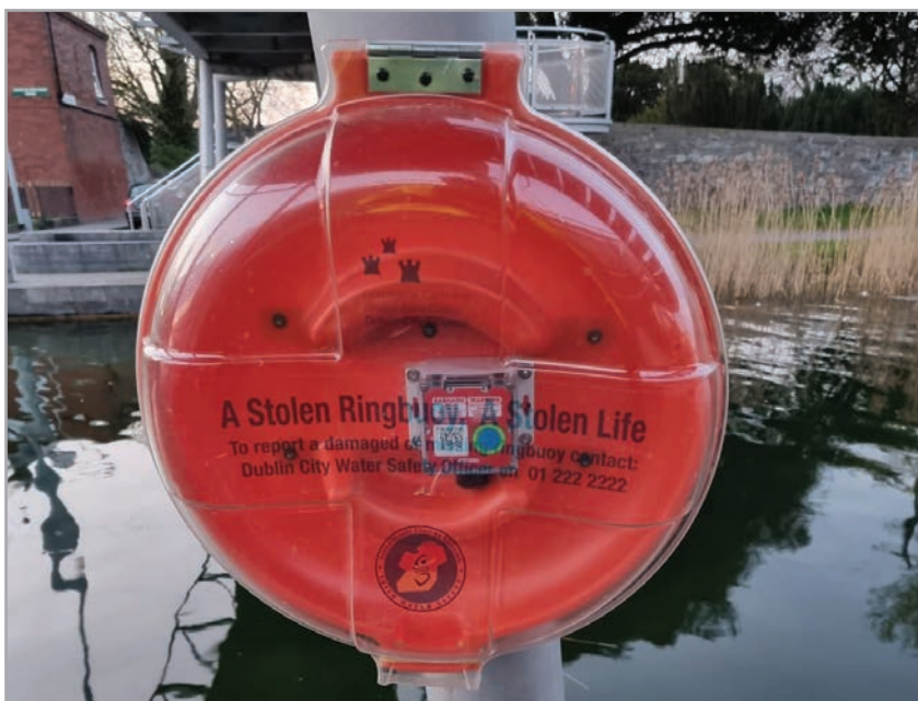
Ring buoy: A sensor is discretely installed to indicate the presence of the ring buoy.
